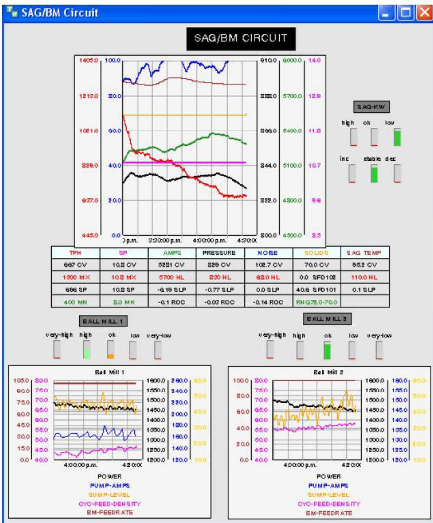
Figure 3. SAG/BM Circuit Expert Dashboard
