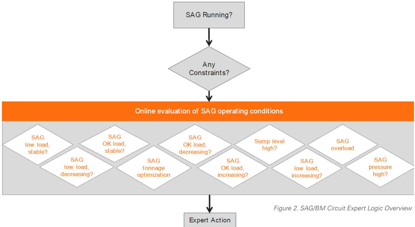
Figure 2. SAG/BM Circuit Expert Logic Overview
