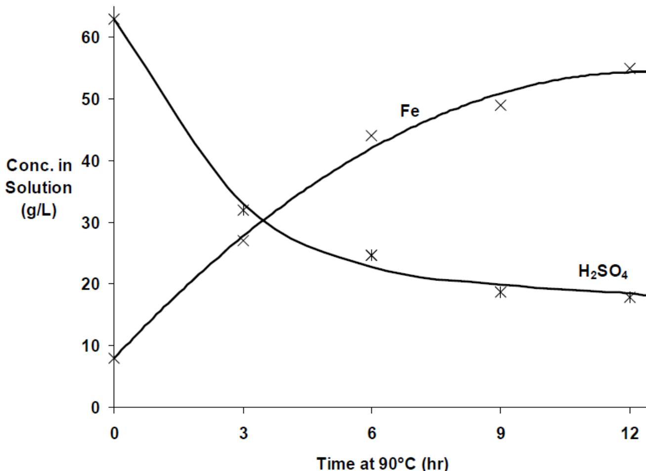
Figure 6 Concentrations of iron and sulphuric acid in solution in the discharge from autoclaving Pueblo Viejo ore, as a function of hot curing time
