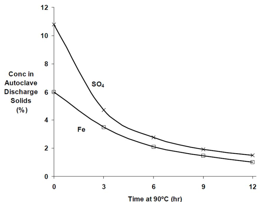
Figure 5 Concentrations of iron and sulphate in the solid residue from autoclaving Pueblo Viejo ore, as a function of hot curing time.
