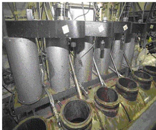
Figure 3 – Continuous Autoclave Agitator Assemblies
