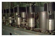
Figure 3: Continuous Autoclave Agitator Assemblies
